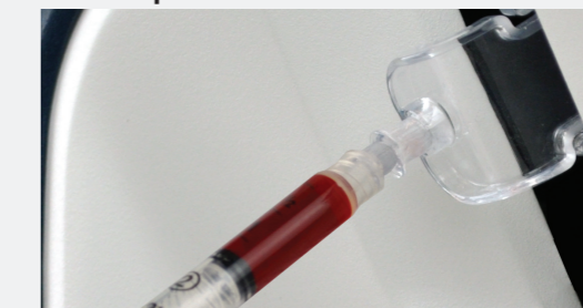
Syringes can be docked and then sampled with hands-free operation.
