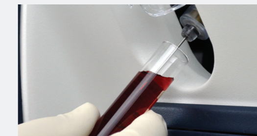
Samples can be aspirated directly from tubes. Sample transfer to a syringe or capillary is eliminated.
