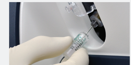
Quality control proficiency ampoules can be sampled without adapters.
